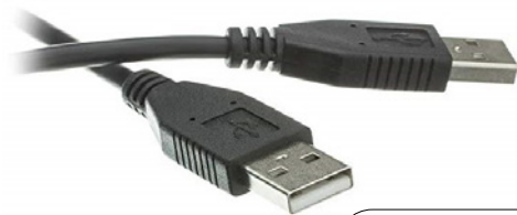
Figure 1: Correct USB Type A Male to Male Connector
